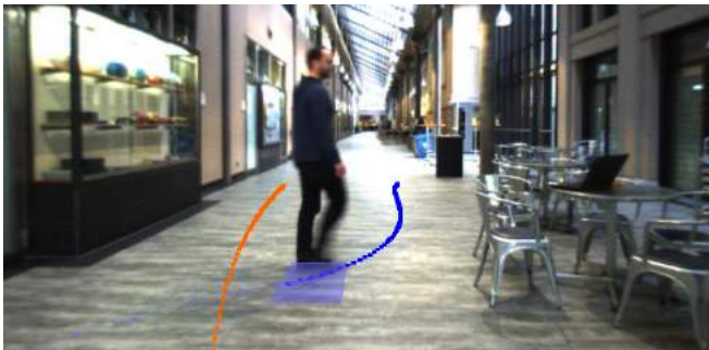
Fig. 2: Predicting the reaction of other agents to static obstacles in the environment affects the robot's plan (orange) too. Based on the typical avoidance distance learned from demonstrations, the robot leaves the pedestrian more room for navigation by swerving to the left.
